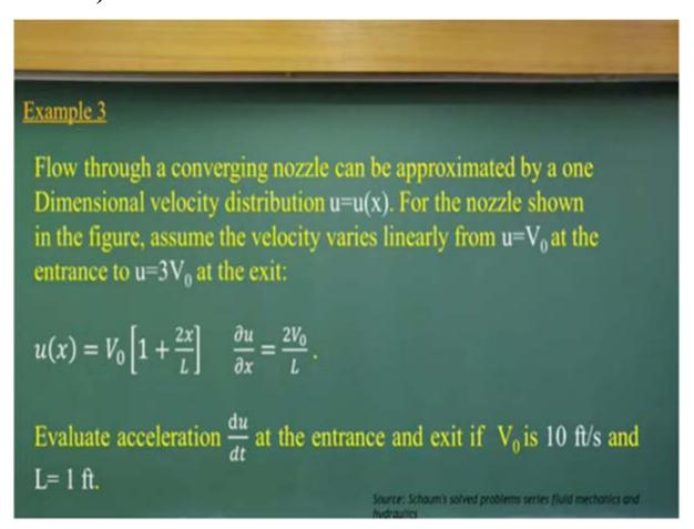
Let us solve the third examples which is a very interesting problems. The flow through a converging nozzle as given in the figure can be approximated as 1 dimensional flow velocity distributions u = u(x) and from the nozzle shown in this figure and assume the velocity varies linearly at this point is  $u = V_0$ .
